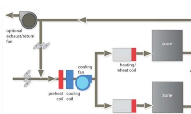
Figure 2. Schematic of modeled system in Trace700
